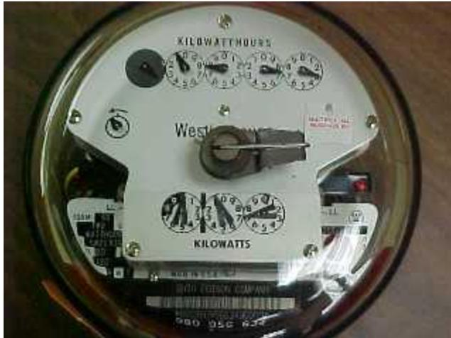
This load meter uses **three small dials**, similar to the electric usage meter, to measure peak load. The vertical black line between the dials indicates the decimal point. Thus, this load meter reads 0.07 kW.
